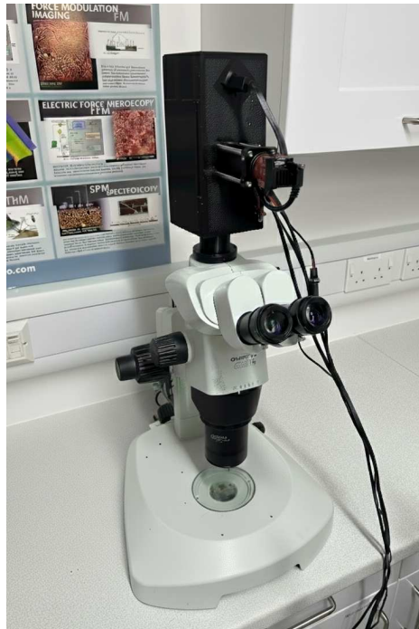
Fig. 6.10 The autofocus device mounted on the Olympus SZX16 stereomicroscope.
